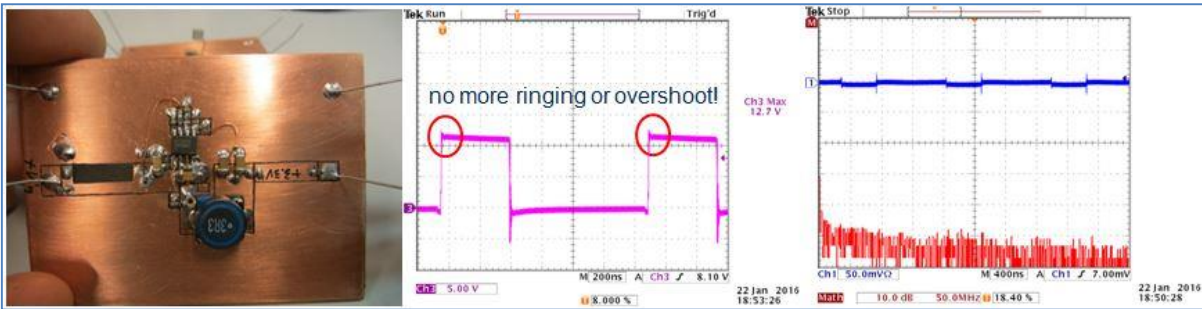
FIGURE 25 : FINAL SOLUTION WITH SHORTEST C_{IN} LOOP
